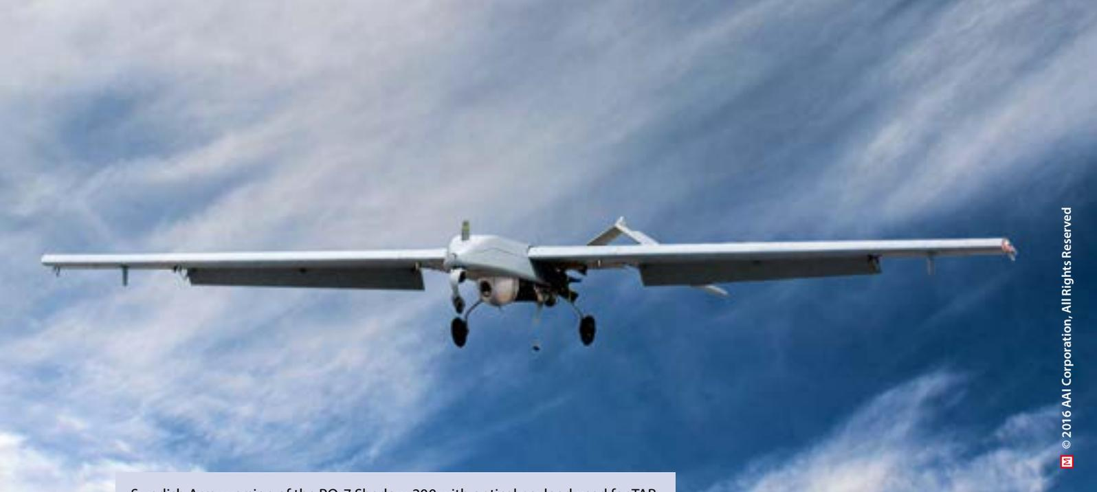
Swedish Army version of the RQ-7 Shadow-200 with optical payload used for TAR.
